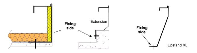
Any other place for fixing may cause water leakage.
