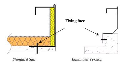
Any other place for the fastening may cause water leakage.
