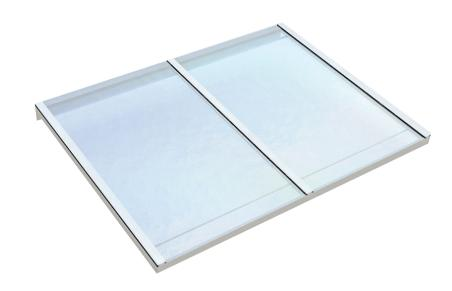
The ARCAPLAN® is a rooflight with a self-supporting extruded aluminium structure, intended for a monopitch roof with a slope of at least 11% (or 6.38°).
